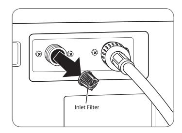
2 Carefully remove the filters from the water valves and soak them in white vinegar or a lime scale remover, following the manufacturer's instructions. Be careful not to damage the filters while cleaning.
